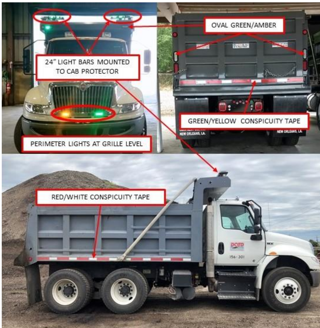
Figure 4 Images calling out location of flashing warning lights on front and rear of truck, and side view calling out red/white conspicuity tape.
