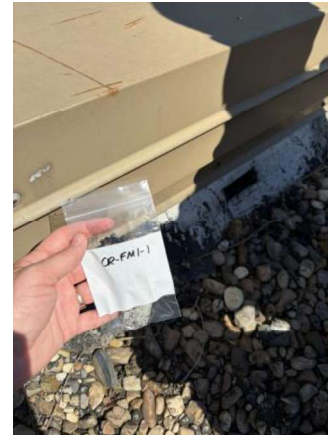
INTERIOR ROOF FLASHING MASTIC (CR-FM1-1, AR-FM1-2, BR-FM1-3)
