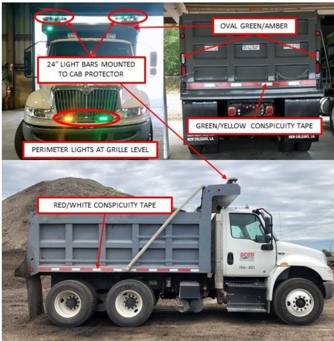
Figure 6: Images calling out location of flashing warning lights on front and rear of truck, and side view calling out red/white conspicuity tape.
