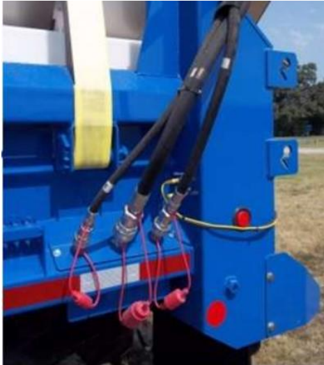
Figure 3: Image of hydraulic couplings mounted to dump bed.
