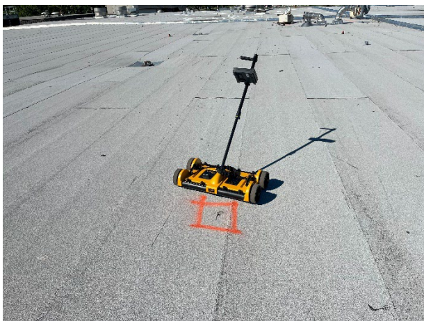
Punctures: no moisture detected
