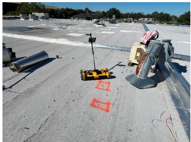
Punctures: no moisture detected
