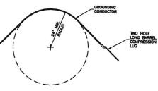
MINIMUM GROUNDING CONDUCTOR RADIUS NOT TO SCALE
