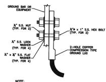
THE SURFACE OF THE EQUIPMENT SHALL BE SANDED DOWN TO THE BARE METAL AND FREE OF ANY DIRT BEFORE APPLYING NO-OX OR EQUAL COMPOUND, PAINT TO MATCH EQUIPMENT.
