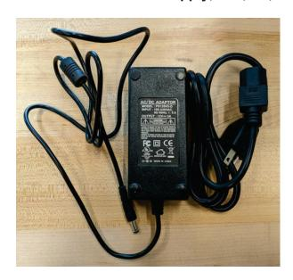
SPECS: 12V, 5A minimum; 2.1mm ID x 5.5mm OD barrel plug
