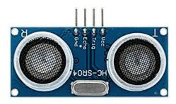
Module: Must have four pins: Vcc, Trig, Echo, Gnd
