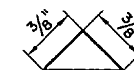
FULL SIZE CROSS SECTION OF 3/8" CHAMFER STRIP TO BE USED IN CONSTRUCTION OF ALL NUMERALS. CHAMFER STRIP FOR SMALL YEAR PLATE
