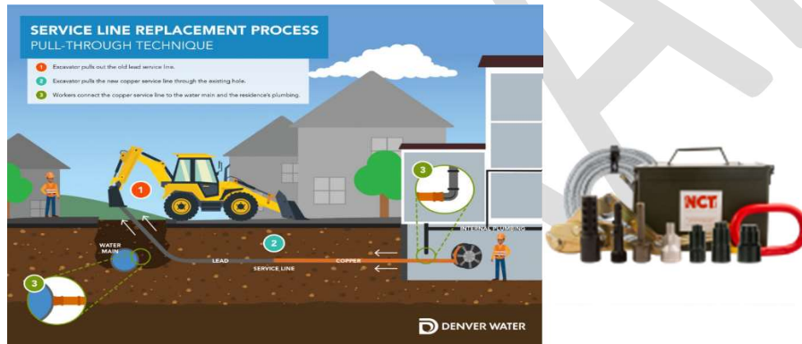
Figure 7.4: Visual of Trenchless -Pull Through Method
