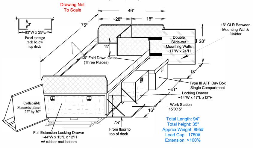
Lower platform is ½" phenolic plywood with 1¾" steel angle rails, hole punched for bungee cord ties. Carrier is also ½" ply, with 1½" angle, also hole punched. 10 ga flattened steel mesh. Drawers Date № 2020 aluminum diamond plate on 500# capacity slides. Decks will have a marine grade textured coating. Steel parts will be powder coated black.
