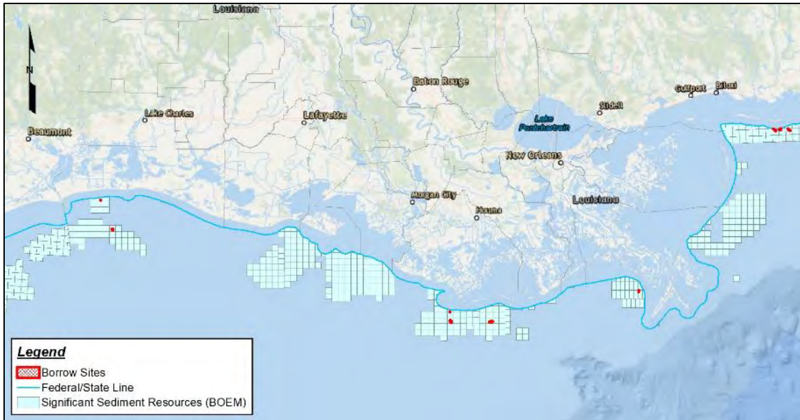
Figure 6. Inventory of borrow sites and OCS blocks designated as significant sediment resources. Because the borrow sites were obtained from MMIS, which is a compilation of data from other sources, some of the borrow sites were originally from CPRA. Note: background is Esri's Imagery Basemap.
