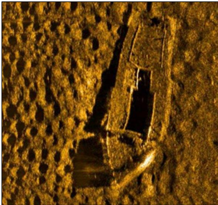
Figure 3. Sidescan sonar image showing a shipwreck and adjacent seafloor, offshore Louisiana in approximately 35 feet of water.
