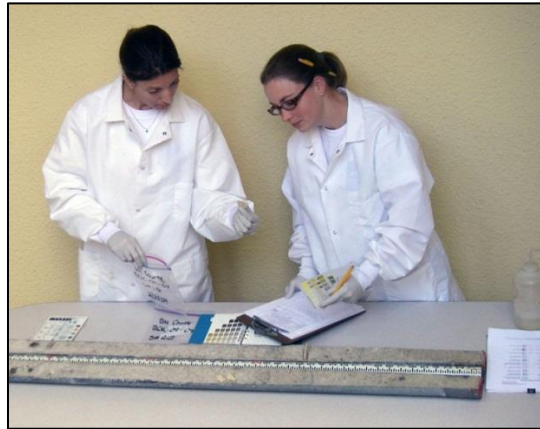
Figure 6. Vibracore logging and sub-sample collection.
