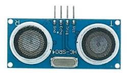
Module: Must have four pins: Vcc, Trig, Echo, Gnd
