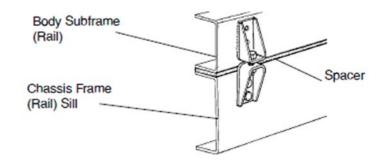
**2.1.2.4.** Fishplate – to be bolted to chassis and bolted or welded to body sub-frame/sill.
