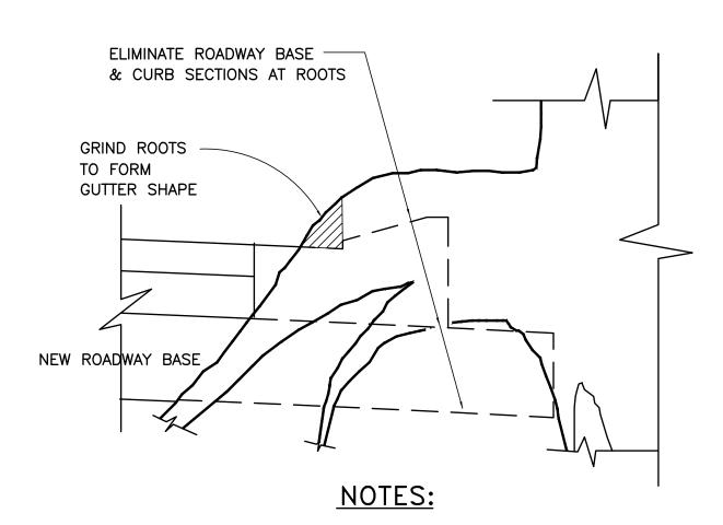
WHERE BIG ROOTS EXTEND INTO ROADWAY SECTION, ELIMINATE ROADWAY BASE AND CURB SECTIONS AT ROOTS, AND GRIND ROOTS TO FORM GUTTER SHAPE MATCHING ADJOINTING CONCRETE GUTTERS AS PER DIRECTION OF THE PKWY. AND PARK COMMISSION.
