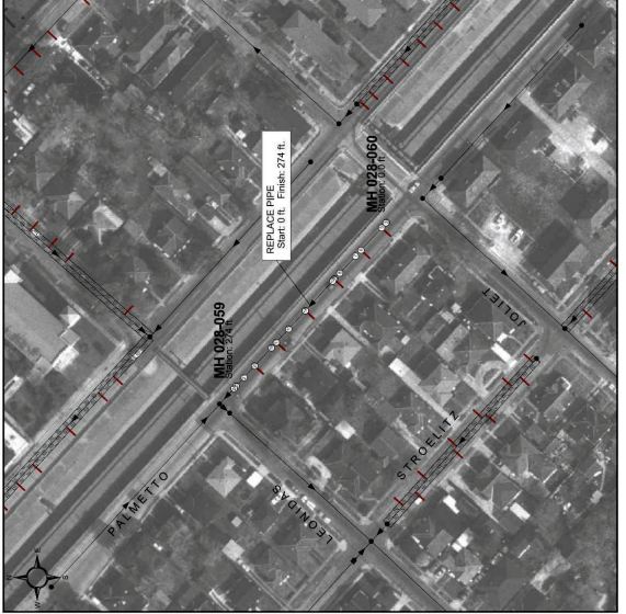
SSERP SEWER REHABILITATION PALMETTO ST (8500) NTS
