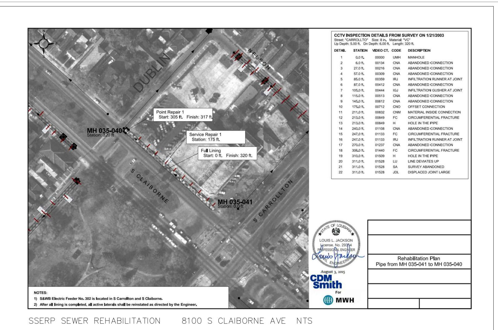
POINT REPAIR 1 (STA 305 FT - 317 FT) RR ASPHALT PVMT = 16 SY SERVICE REPAIR 1 (STA 175 FT) RR ASPHALT PVMT = 14 SY RR CURB = 8 LF RR SOD = 3.6 SY RR CONC SW 4 INCH = 3.6 SY
