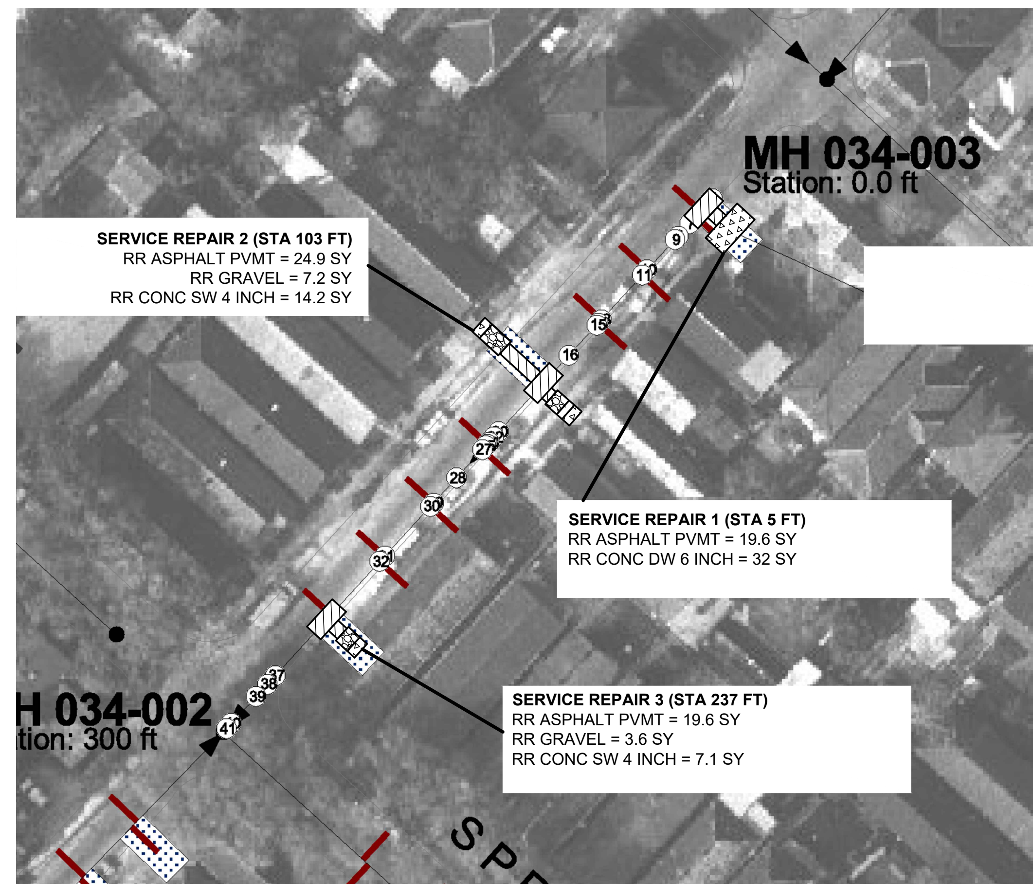
SSERP ROADWAY RESTORATION CAMBRONNE ST (2000) NTS
