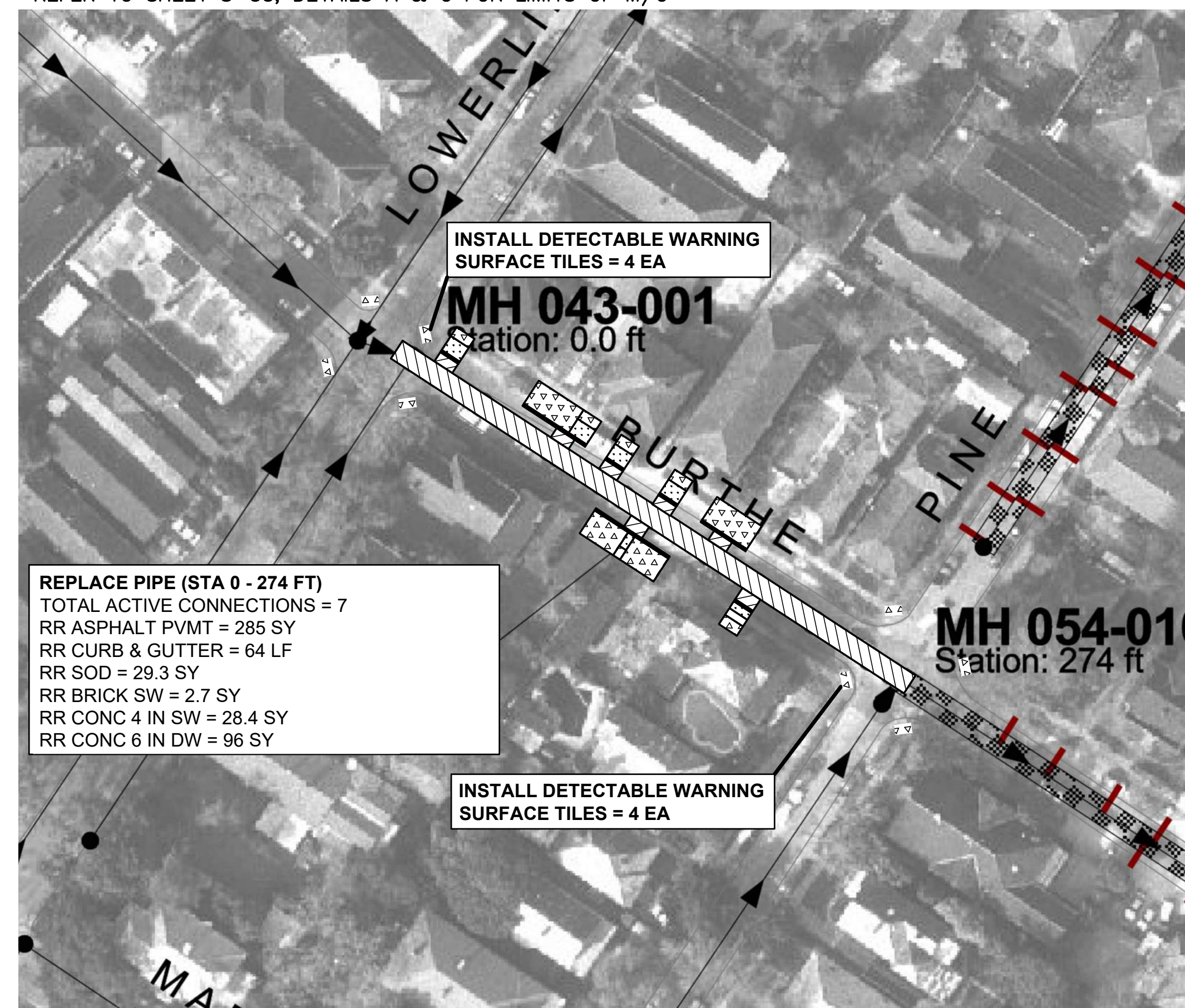
SSERP ROADWAY RESTORATION BURTHE ST (7300) NTS
