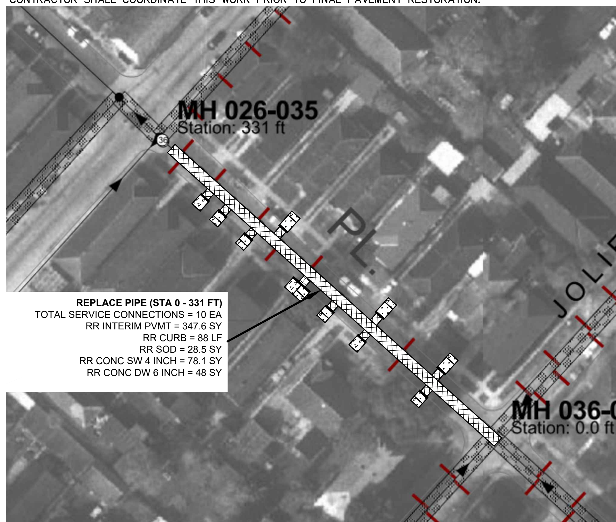
SSERP ROADWAY RESTORATION PRITCHARD (8500) NTS
